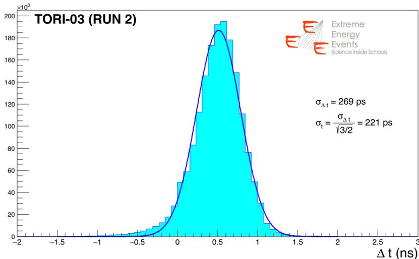
$\Delta t$  distribution for one of the EEE telescopes (TORI-03), showing the gaussian fit and the time resolution
