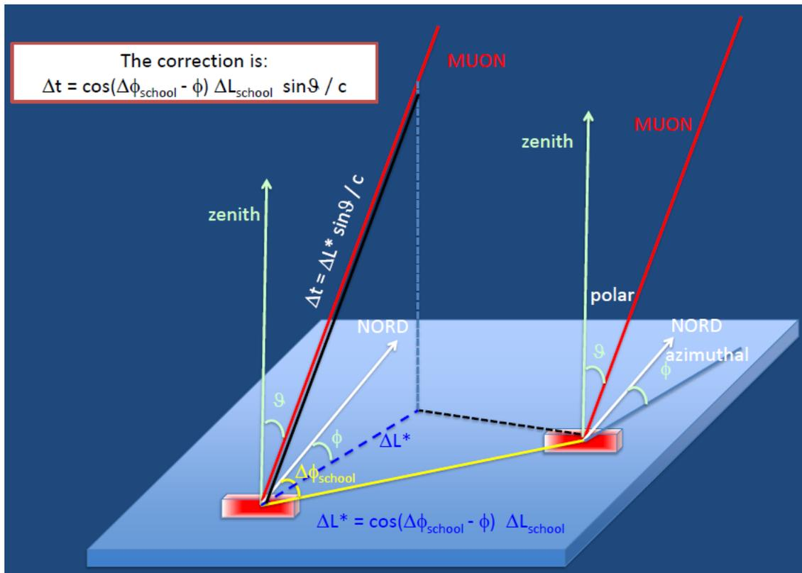
EEE telescopes allow to reconstruct the direction of the shower secondaries, i.e. of the **shower axis**
