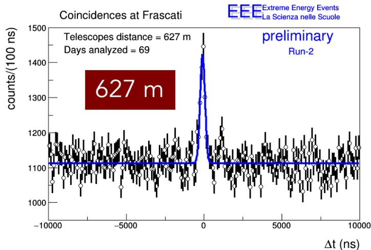
The width of the reconstructed peak is usually of the order of **200-250 ns** (CERN and Bologna cases differ because of particular GPS setups)
