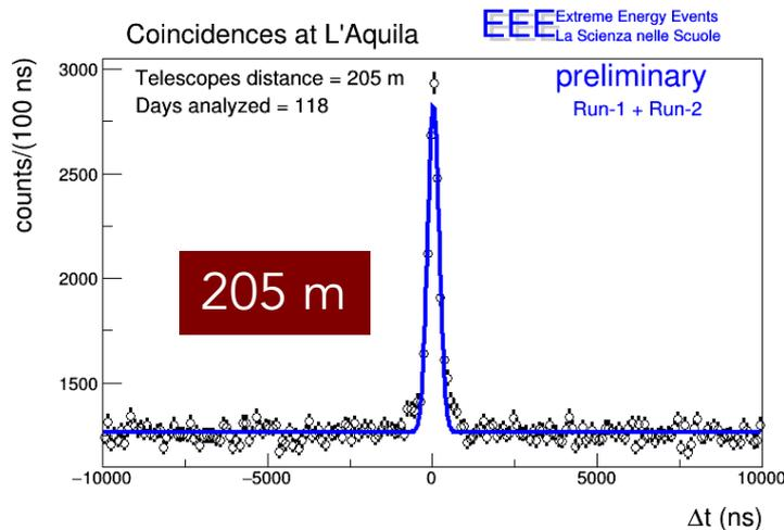
Single-track coincidences between 2 telescopes were well reconstructed for several distances between telescopes
