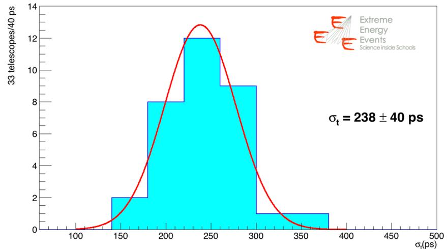
Time resolution measured with data taken in Run 3, for 33 telescopes: the average time resolution is given by the gaussian fit and is  $\sigma_t = 238 \text{ ps}$
