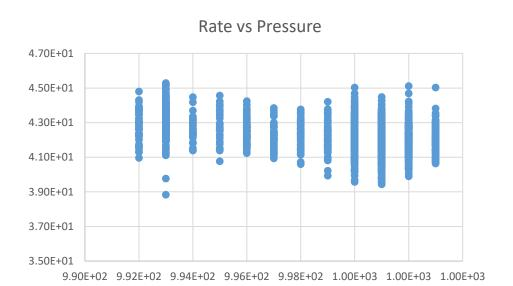
It is quite difficult to appreciate variation in the flux in a scatter plot because of the large fluctuations (the statistics of each point corresponds to 1 minute of data acquisition)
