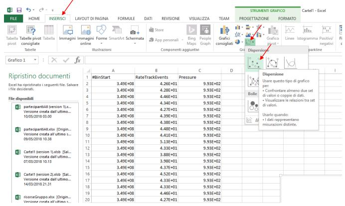
We can start by inserting a graph showing the trend of the track rate vs pressure
