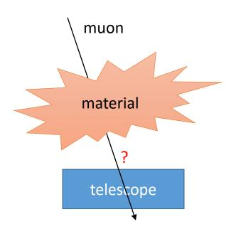
If we put some matter in front of our telescope the muon may be absorbed during its propagation in the material  $\rightarrow$  we expect to reduce the arrival probability to the telescope.
