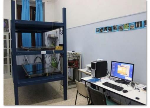
The track is the result of the crossing of muons through the three chambers. Using three impact points (one on each mrpc of the telescope) it is possible to reconstruct the direction of the crossing muon, obtaining then the ZENITHAL ANGLE.
