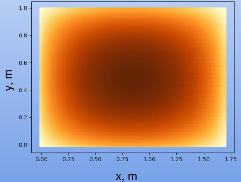
We have written a program, which goes through all possible tracks directions, generating parametric quantity of random dots on the imaginary layer (which is bigger than a chamber and located above the telescope) and counting differential geometric efficiency.
