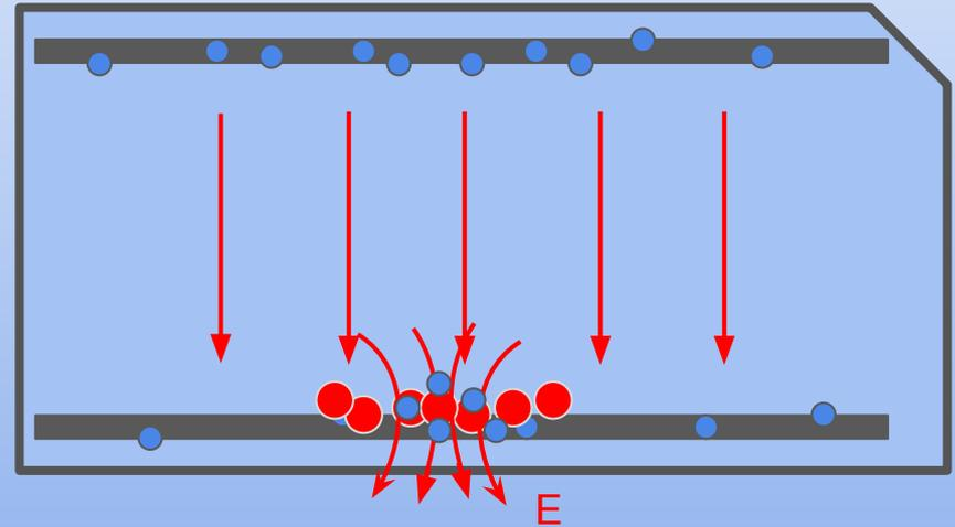
Our hypothesis: after positive ions accumulated on the dielectric surface they create a strong double-layer electric field which cause emission of electrons, but not single, but in form of electron busts , Such bust were first observed in vacuum breakdowns and then also observed in the case of gaseous detectors
