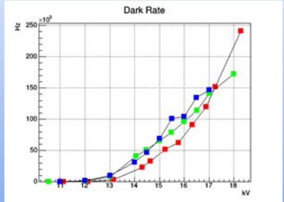
Dark rate – frequency of random electric impulses on the electrode, that does not linked with with incoming particles
