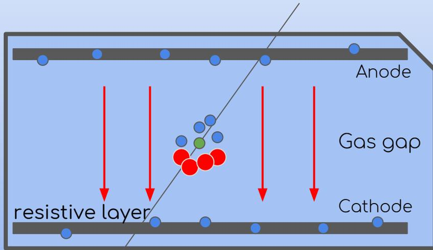
Malter Effect represents emission single electrons from cathode. Published mathematical model of those effect was based on Zimerfiled theory of field emission. Because of, the classical Malter Effect predicts single electron emission, one can speculate that it can not be observed in RPC due to the small avalanche charge.
