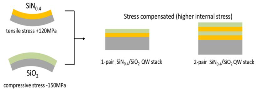
SiN<sub>0.4</sub> /SiO<sub>2</sub> QW pairs deposited by all-CVD process show room temperature mechanical loss  $\sim 10^{-5}$ , lower than Ta<sub>2</sub>O<sub>5</sub> -TiO<sub>2</sub> /SiO<sub>2</sub> in current GW detector.
