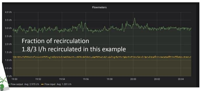
At present the prototype can reaused a flow fraction ~60%
