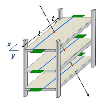
The impact time in each MRPC is reconstructed as the average of signal arrival times at the strip ends (RIGHT and LEFT SIDE)
