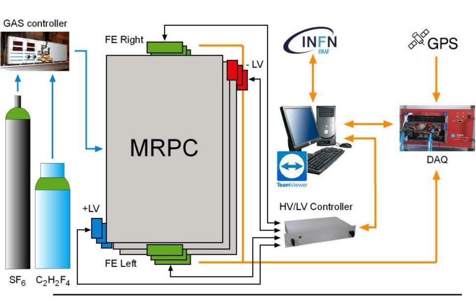
3 Multigap Resistive Plate Chambers (MRPCs) for tracking particles
