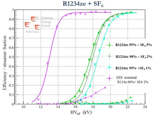
SF<sub>6</sub> is a very effective quencher also in a small percentage , but due its very high GWP value (GWP = 23900) , its fraction should not exceed 0.5%
