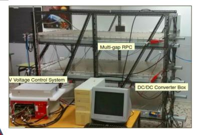
A chamber is accepted if the leakage rate at  $\Delta P_{atm} \sim 1$  mbar is lower than the maximum value: 0.1 | /h
