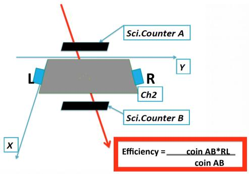
The values of working voltage efficiency with scintillators were:
