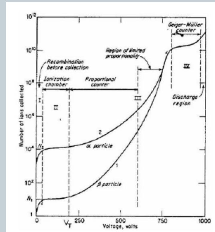
In the proportional counter region the function that describes the gas coefficients is similar to the t.o.t. function obtained from experimental data.
