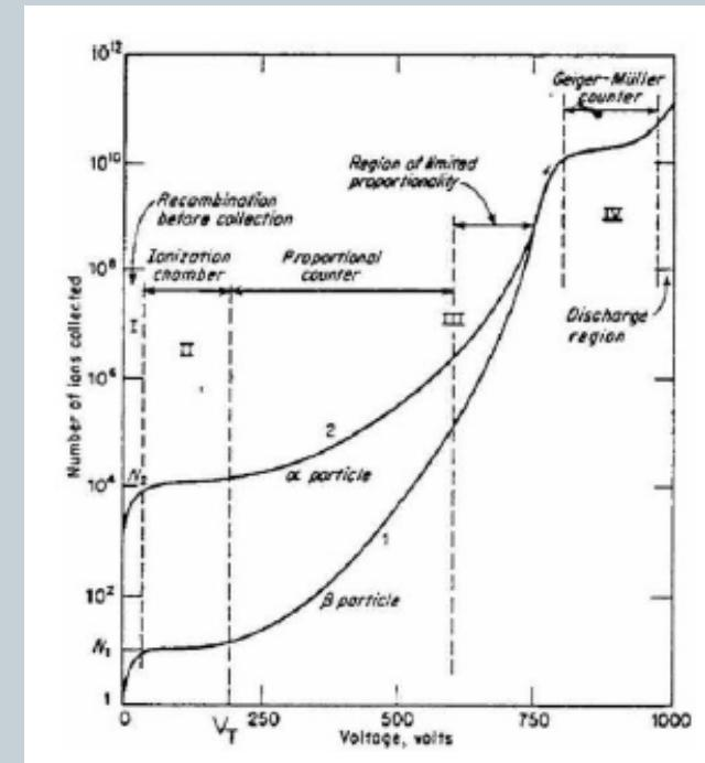
The collected charge also depends on the gas and on the intensity of the electric field; our detector operates in the proportional counter.
