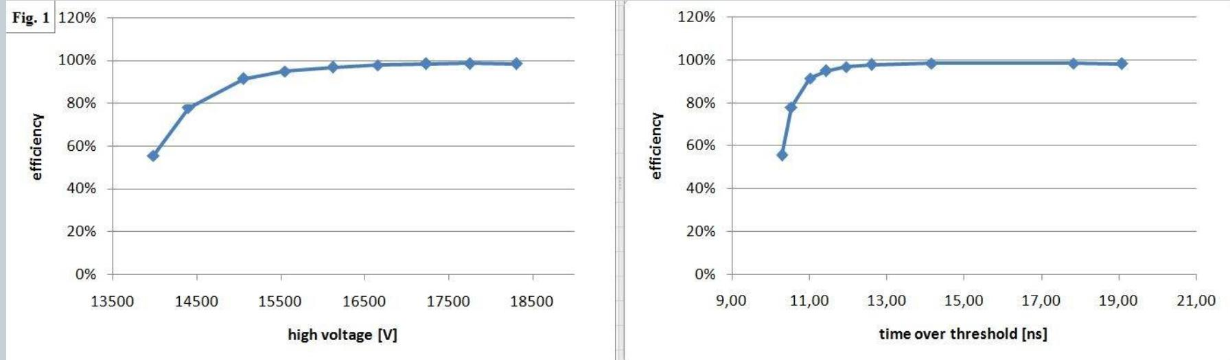
The efficiency tends towards 98% while the t.o.t. grows, as it does with the high voltage.
