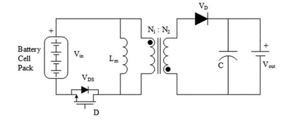
The figure shows a basic schematics of a DC-DC converter: an input DC voltage is transformed to AC with an oscillator (a mosfet in this example) and then applied to a transformer. The output voltage is then rectified with a diode and filtered by a capacitor. The ratio N2/N1 of the transformer coils determines the ratio between Vout and Vin.
