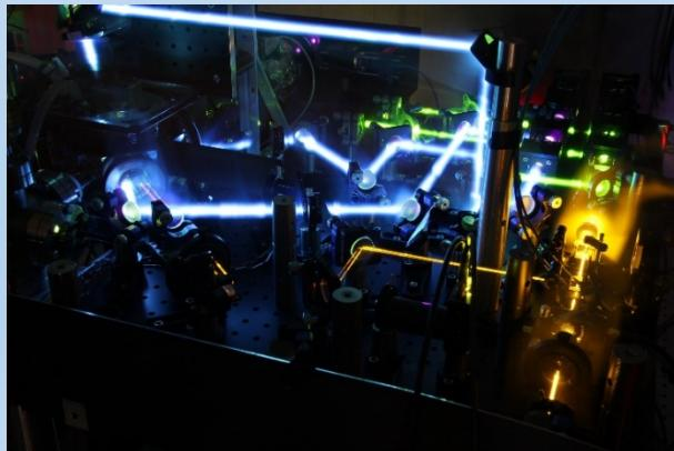
In an ytterbium optical clock, the frequency of an ultra-stable laser is locked to a particular transition of ytterbium prepared in an ultra-cold atom sample
