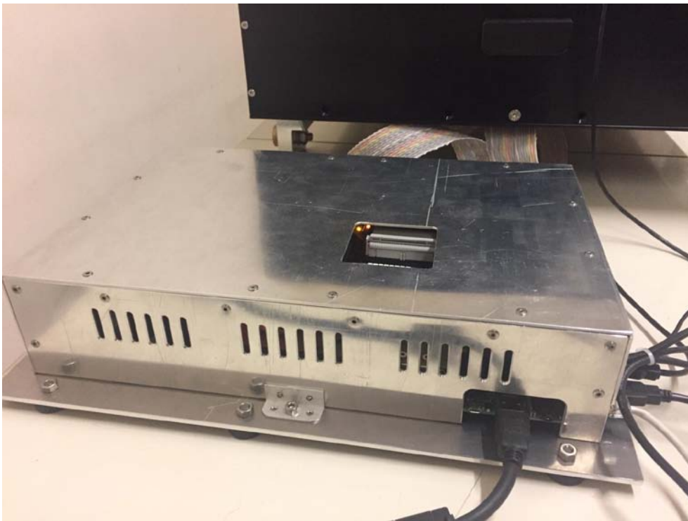
Figure 2: Detail of the box hosting the readout electronics of one of the PolarquEEEst detectors; in this case the box has been detached from the main bulk and placed aside.
