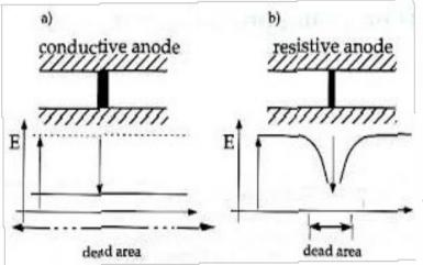
They replace conductive planes and guarantee the localized spread of charges. In this way, the charging time of the electrodes is about 1 ms, so there is a minimum tension which is restored directly from the power supply system. In this way the telescope does not need an external shutdown circuit.
