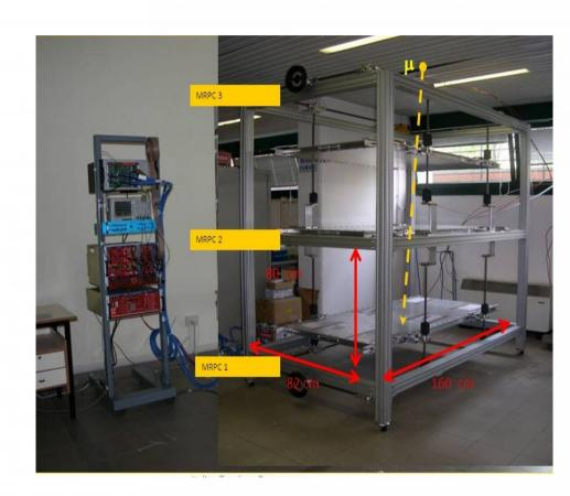
Resistive electrode chambers in which is enclosed a mixture of Freon (98%) and sulfor hexafluoride (2%).
